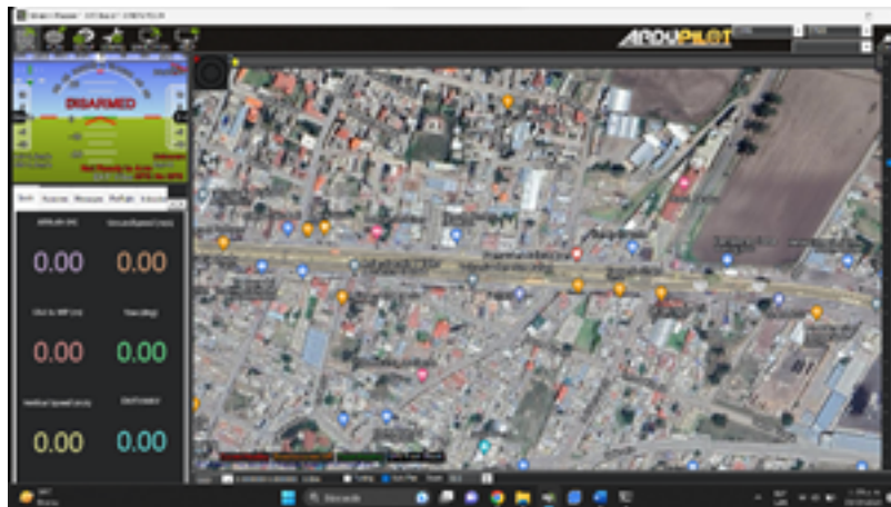
Figura 2: Interfaz Principal del Software Mission Planner.
